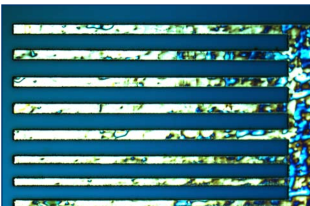
Material amorphous metal Laser femtoREGEN™ \tau = 350 fs \lambda = 1040 nm
