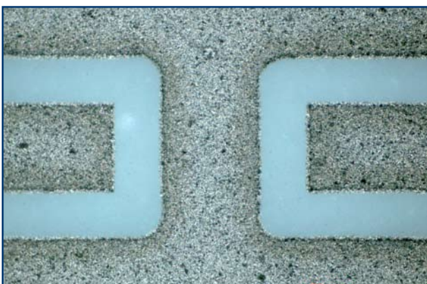
Material silver on ceramics Laser femtoREGEN™ \tau = 350 fs \lambda = 1040 nm
